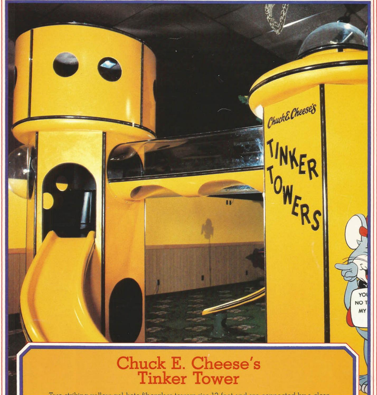
Two striking yellow gel-kote fiberglass towers rise 12 feet and are connected by a clear plastic crawl tube. Each tower has a four foot high curved slide. Comes complete with its own sound system featuring circus music and bright, happy chaser lights for maximum visibility. Great for little kids.
