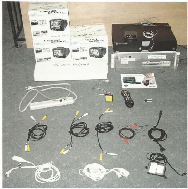
In the Tivo Box, you will find 3 stereo RCA cables and one Single Conductor. Also, you will find the power cord for the Tivo, 2 short extension cords to plug the Wall Warts into. A multiple Outlet Strip to plug the Tivo, the Tivo Controller, and the two extension cords into which are powering the 3 Wall Warts for the monitors and the one Wall Wart for the AGFM DC Input supply. You will also find the AGFM DC Wall Wart. The Monitor Wall Warts are in the boxes with the monitors.
