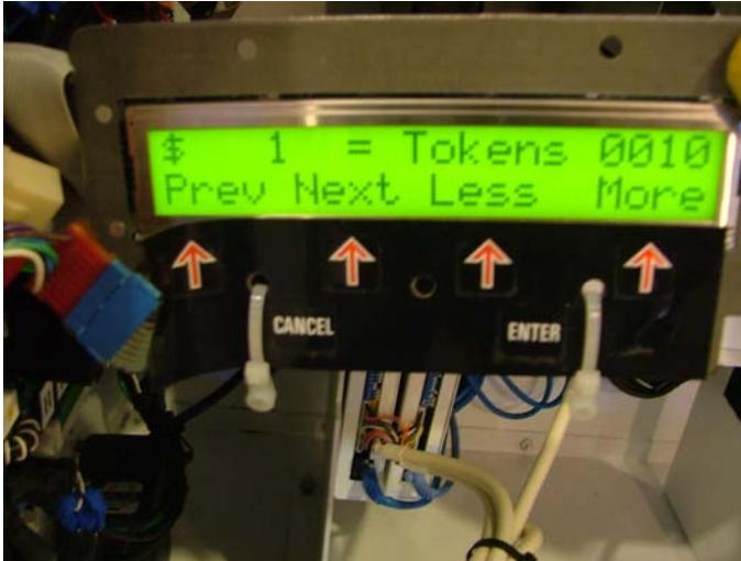
Note: Since both the 10 Token and 20 Token controllers use the same credit wires, you will need to set the 20 Token controller to 2 Pulses.
