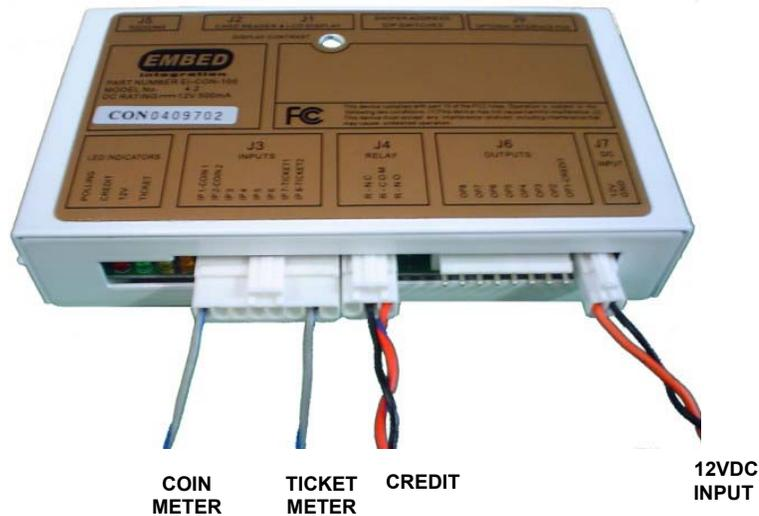
14. Through an existing opening in the rear of the machine run the RJ45 patch cable through to the controller and plug into position J5. Where no opening exists you will need to drill a
