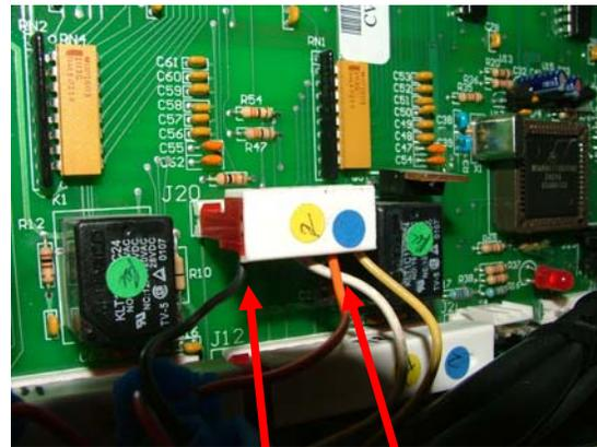
Attach credit wires from 1 token Swiper here.
