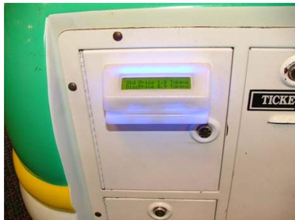
**Tri Door Coin Mechanism with Swiper holes (pre-drilled)**
