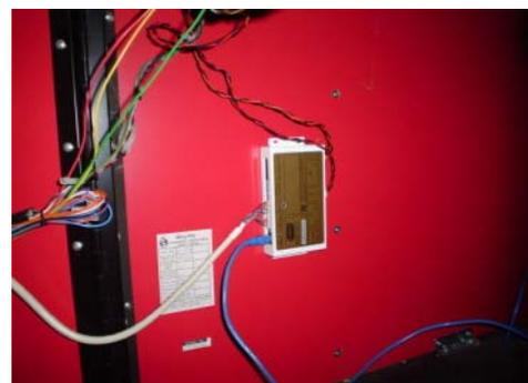
controller and harnessing be installed as far away as practical from any sources of EMI, i.e. motors, relays, SCR switches. Connect the swiper cable to J1 and J2 on the Controller.
