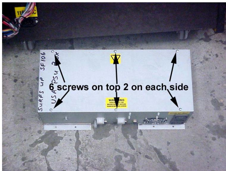
Remove the cover of the power supply and locate the two toroidal (circular) transformers in the left side of the power supply.
